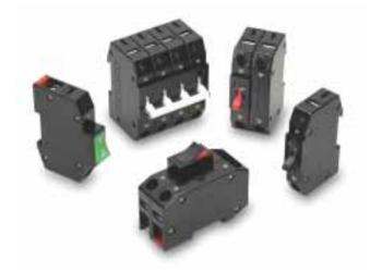
Designed for snap-on-back panel rail mounting on either a 35mm x 7.5mm, or a 35mm x 15mm Symmetrical Din Rail, allowing rapid and simple mounting and removal of the breaker. It features recessed, wire-ready, touch-proof, shock-resistant terminals, suitable for automatic screwdriver assembly, as well as "Dead Front" construction characteristics.
